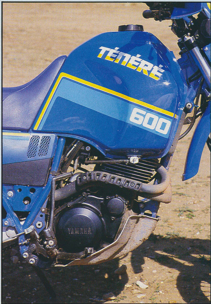
The '86 Tenere's tank looks bigger than last year's but it's actually six litres smaller at 23 litres (5.06 galls). Power unit (what you can see of it) is externally similar but it's been tweaked for another three bhp.
