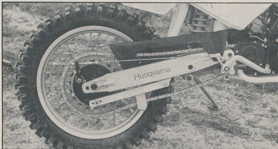
Chain tensioning is a simple task, but adjusting the brake lever height is slightly more time consuming. Note the safety-wire on the lever.
