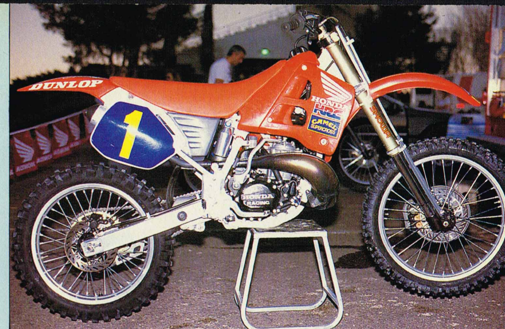
Top riders adjust their chassis for individual tracks to get the most from their machine. Here Jeff Stanton has moved his rear wheel as far back as it'll go and dropped the forks to their minimum height for more stability. On a tight track, raise the forks in the triple clamps and shorten the wheelbase.
