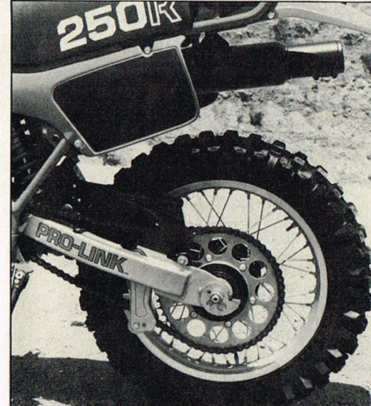
The Pro-Link rear end is just about the best thing that could ever happen to the XR. We were happiest with the damping on the #3 setting.
