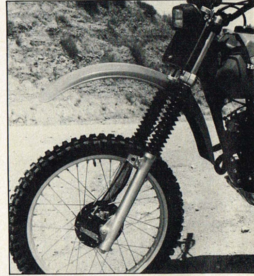
Air/spring forks are new for this year; so is super-strong double-leading shoe brake system. So far, we've heard no complaints about the change to 21-inch front wheels.
