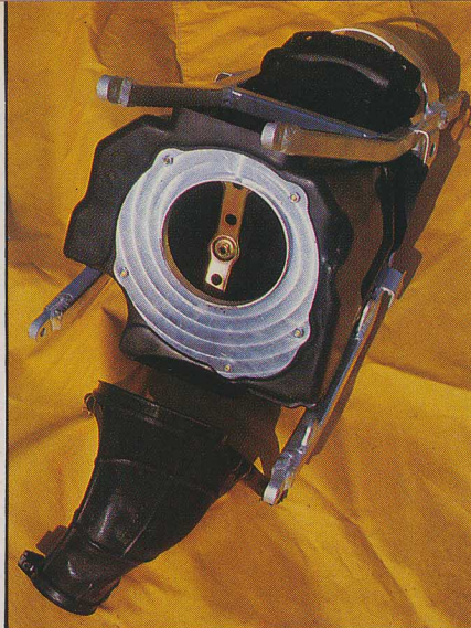
A handmade aluminum subframe, cradling a Honda CR250 airbox, will be fitted to both ISDE DRs. Hours of measuring and fabrication result in lighter weight and longer filter service intervals, vital for continuous ISDE riding.
