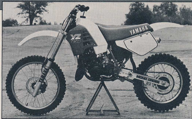
Lots of changes for '86: The newest YZ250 sports a low-sided, low-center-of-gravity fuel tank; a new, smaller disc brake; improved suspension; a new chassis (10mm longer); better clutch and shift action and better tires.
