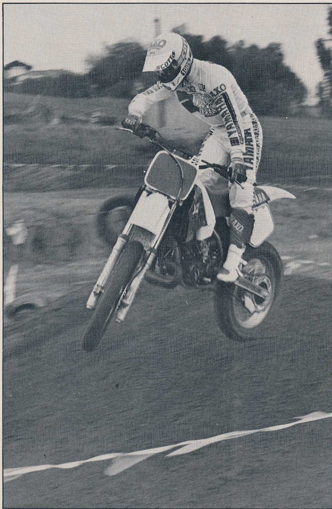
Yamaha's Ohlins-designed rear shock is a drastic improvement over the '85's pogo-spring device. Ergonomics have been improved as well—the YZ's seat/peg/bar relationship is correct for more people this year. The new, lower tank allows for more weight transfer in the corners and makes for easier air-time maneuvers.
