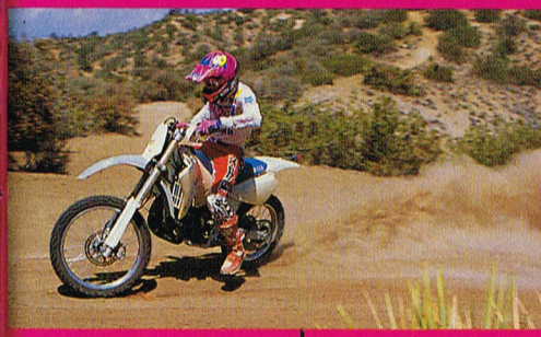
Damon Bradshaw tests the speedway capability of the 1991 WR200. Basically a DT200 in a YZ chassis, the WR200 can change from a hare scrambles mount to a competitive enduro bike with the addition of a roll chart holder and/or computer. It has more suspension than a KDX200 . . . and a taller seat height.
