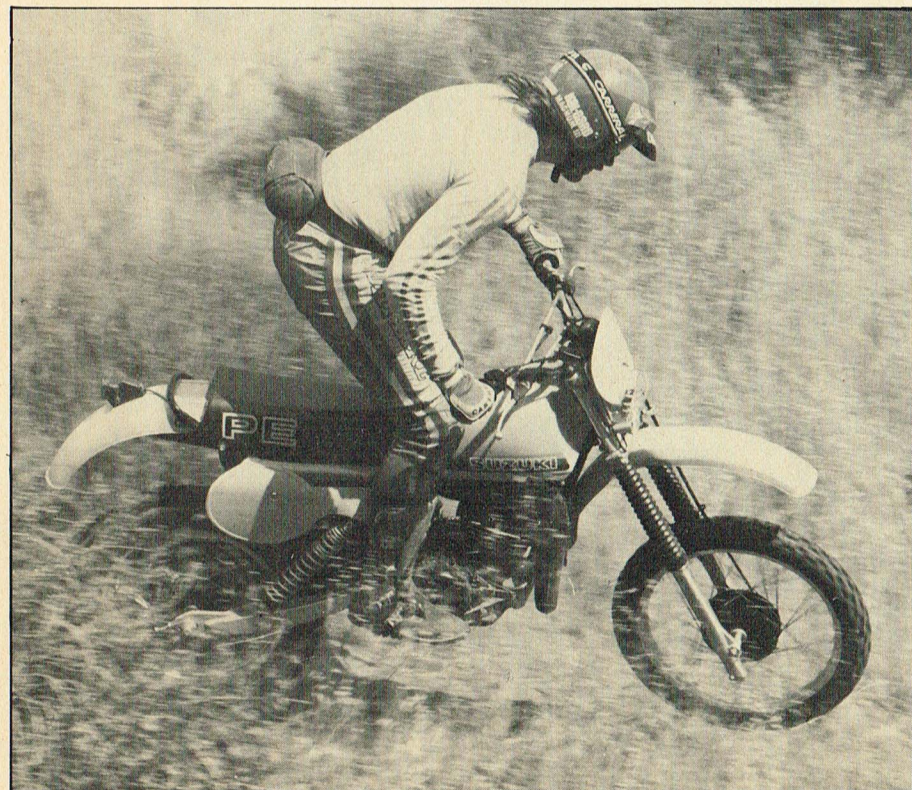
Both the front and rear suspensions aren't up to par with the competition's. The forks are skimpy 36mm models and the shocks are antiquated compared to the deluxe Ohlins and Fox shocks.
