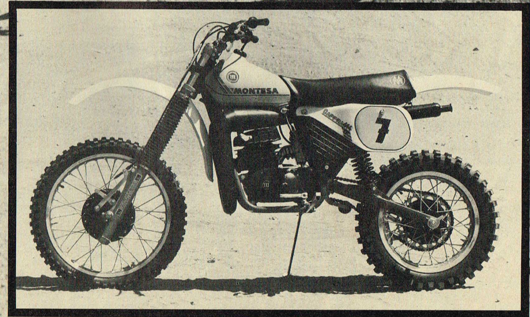
Sitting very tall, even for a new-generation, long-travel bike, the 414VG has a short wheelbase. The combination of these two things makes directional changes easy, but this sacrifices high-speed stability over rough tracks.
