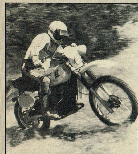
An Answer Products spark arrester saves weight while keeping down the decibels. The seat cover adds a nice touch.
