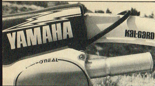
An Answer Products spark arrester saves weight while keeping down the decibels. The seat cover adds a nice touch.
