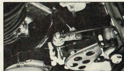
Extending the clutch arm 3/8 of an inch makes the action much easier.
