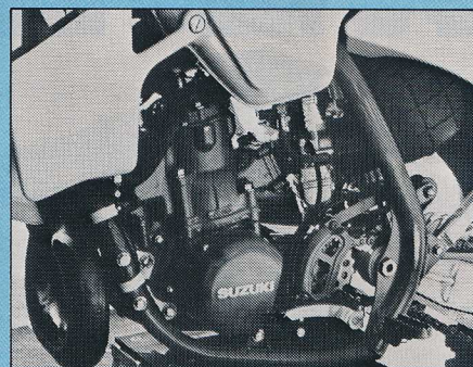
Suzuki concentrated on giving the 1988 RM250 a harder hit and a longer pull through the power curve. Carburetion is by the new flat-slide Mikuni TM mixer. A two-piece clutch cover might show up on the production bike.
