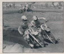
Cornering the YZ360 is much easier than the KX500, but the YZ isn't as stable on the straights, especially in sand. The full 500s accelerate faster but also tire the rider faster than the lighter 360.
