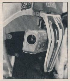
Torque is increased with the 360cc kit and we further enhanced low- and midrange with Answer's new Variable Flow Control muffler, which increases back pressure at low revs and decreases noise output (Dec. '88 DIRT BIKE).
