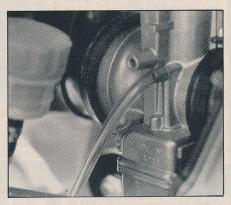
An '88 YZ250 intake manifold and reed assembly are needed to convert the '89 YZ and we had trouble with our airbox boot pulling off of the carb until we replaced the wimpy stock clamp with an automotive hose clamp.
