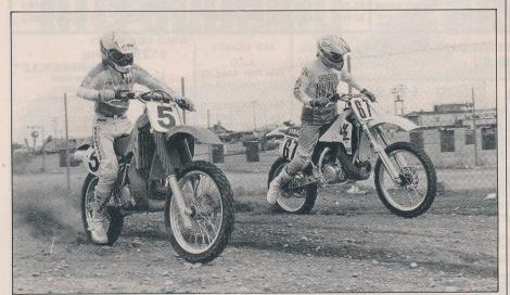
Drag-racing the YZ360 and KX500 ten times resulted in six KX wins to the 360's four wins. On top-end (with stock gearing) the KX500 will run away and hide but the YZ holds its own on short-start straights and on tight tracks.
