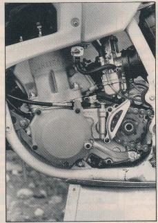
Where the 250 power valve acts as the top edge of the exhaust port, the 360 setup is like a booster port. A pencil-sized rod that has an elongated port through its length blocks a booster port above the exhaust port. When the revs build, the rod turns and "opens" the sub port, effectively raising port height.
