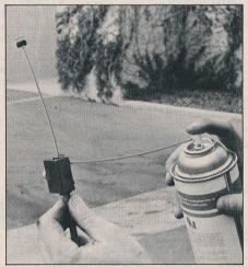
Properly lubricated cables are a must with KTMs. Not only will the cable work better, it will also last longer. Z Racing recommends lubing the cable after every race.
