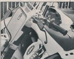
Another trick for KTM clutches is to install a Honda CR lever and perch. The design and action of the Honda lever/perch combination is superior to the stock KTM assembly.
