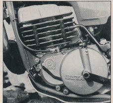
Beta completely reworked the clutch for '88. A new basket, actuator system, metal plates, cork plates and a larger cable considerably improve clutch action. Other than that, the lower end of the six-speed, primary-start motor is unchanged. Highquality parts, such as needle transmission bearings, Motoplat ignition and Boyesen reeds, abound.
