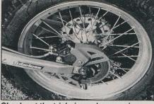
Check out the trick rim and magnesium hub; the spoke nipples ride in the hub to simplify sealing the rim for the tubeless Michelin rear tire, which is the industry standard. The rear brake is more powerful. thanks to a new master cylinder, but debris in the system fouled the brakes on our test unit. Flushing the system solved the problem.
