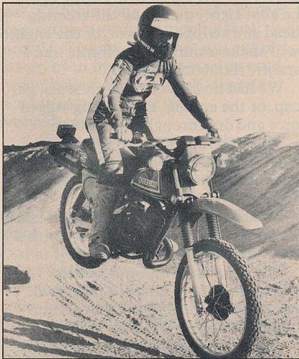
As with most dual-purpose motorcycles, the forks were too soft for the whoops, and the rear end hopped around to boot.
