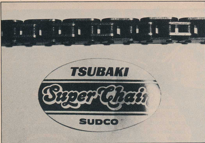
When your old chain looks like this, it's time for a new one. From here, it will not only wear out even worse, but can ruin both sprockets as well.
