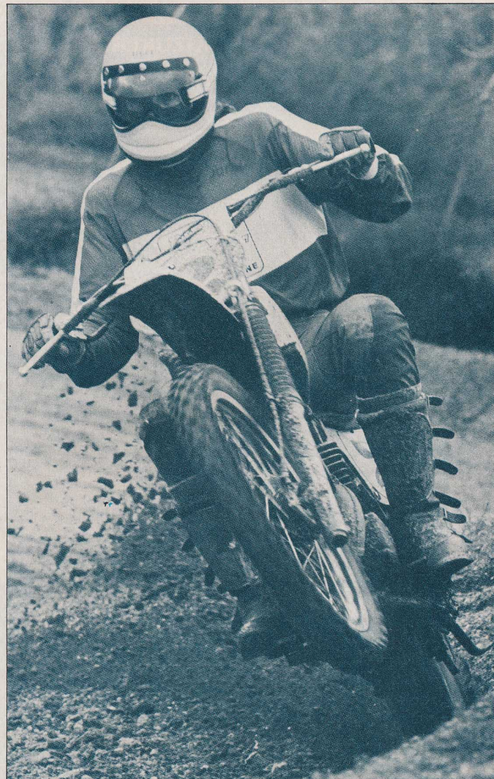
The C's long legs are similar to the 250C's, but have improved dampening and spring rates, and more air volume with the tall aluminum air caps.
