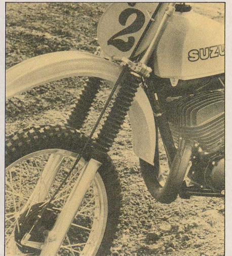
The C's long legs are similar to the 250C's, but have improved dampening and spring rates, and more air volume with the tall aluminum air caps.
