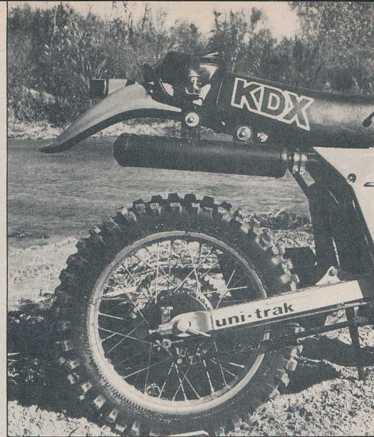
Rear end sports new "Uni-Trak" stickers, and otherwise remains the same. Rear brake arm can take a lot of abuse from rocks, without breaking.
