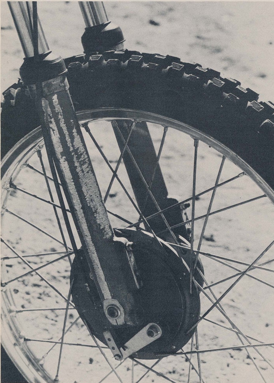
Fork legs are home-cast magnesium. Allen head bolt on each leg adjusts damping.
