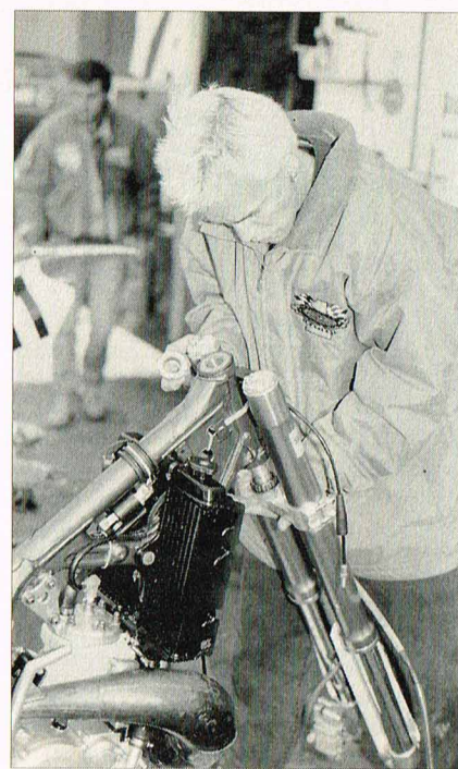
The works Kayaba fork and YMU billet aluminum clamps make the flight already assembled. Even the factory front brake m/c, line and caliper are installed.
