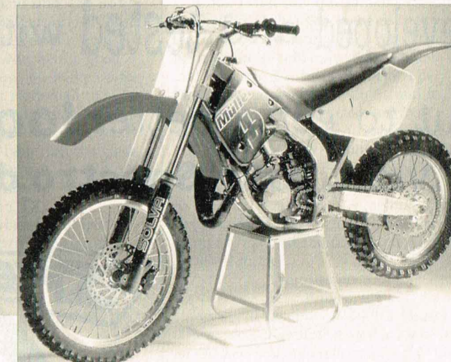
Three years before Honda released the aluminum perimeter-framed CR250R, Müller was selling its own aluminum MX125. The Müller sports Talon hubs, billet clamps, a Solva conventional fork, Ohlins shock and a 38mm PWK Keihin carb. Call (941) 566-9666.
