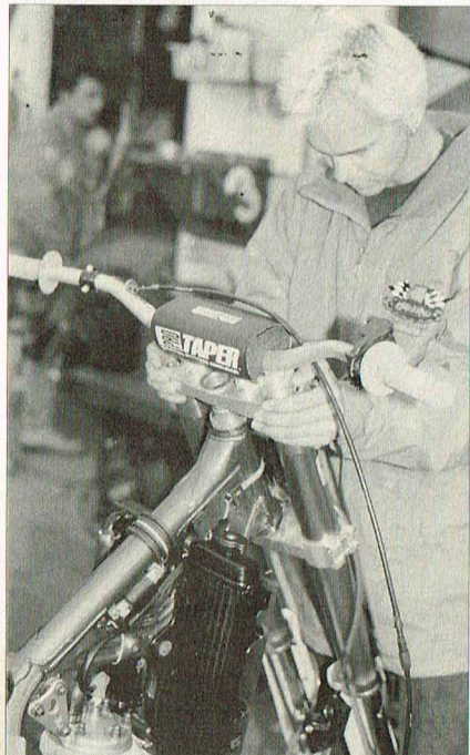
Although Jeremy didn't bring a Ti sub-frame, Randy had to replace the stock one with one shortened to provide a lower seat and rear fender. He replaced the air filter with a UNI.
