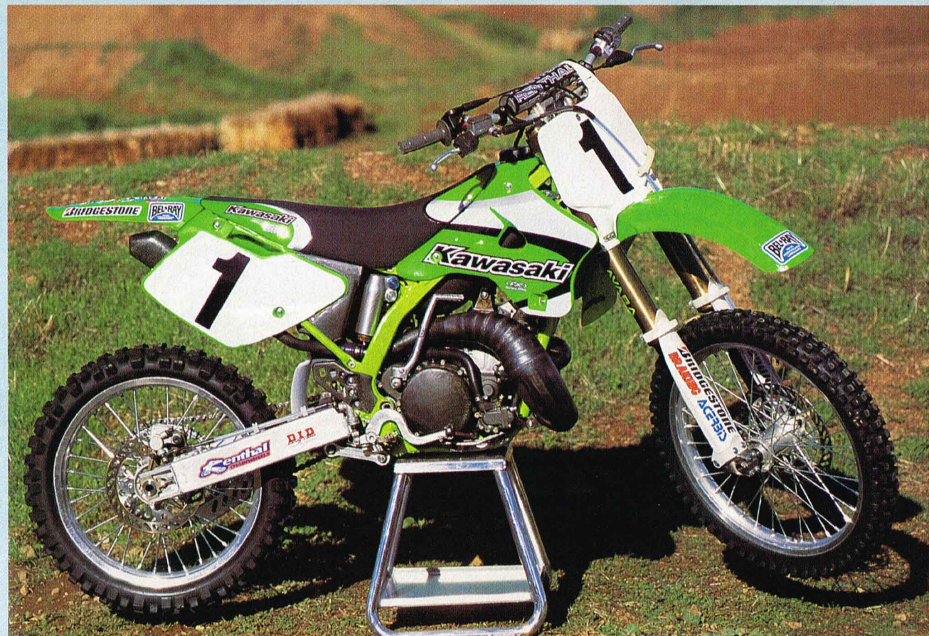
Top: Right up until the Coliseum opener, Team Kawasaki was refining settings. Berg Racing carbon-fiber pieces mount the fork canisters to the upper tubes, and Kawasaki has developed an external canister for the shock, too. There is also a new throttle-position sensor for the traction-control circuit of the ignition.
