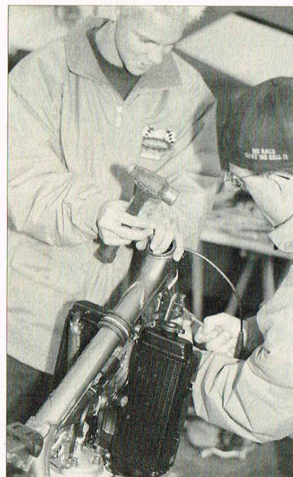
Lawrence removed the stock fork assembly, then drove the lower headset race out of the frame. Jeremy's works fork assembly uses a different lower bearing, so a new race was mandatory.
