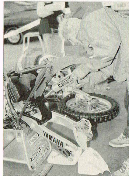
Although Jeremy didn't bring a Ti sub-frame, Randy had to replace the stock one with one shortened to provide a lower seat and rear fender. He replaced the air filter with a UNI.
