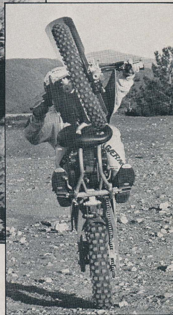
A look at the undercarriage provided by wheelie expert Steve Schmitz shows a highly vulnerable pipe. We dented ours in a semi-slow front-end wash out. ►
