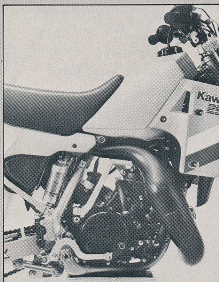
Power forms at the bottom with the '87 KX and surges into a strong mid-range. A change in the stroke, as well as some head mods, let the Kawa dig trenches and climb virtually anything.
