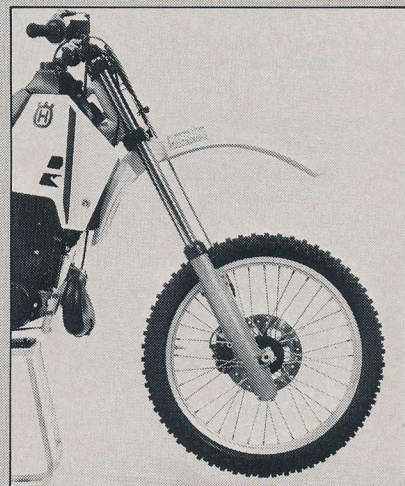
Don't write off the forks. They still flex, but the damping has been greatly improved and once we installed the Progressive springs, we felt it damped as well as any forks around.
