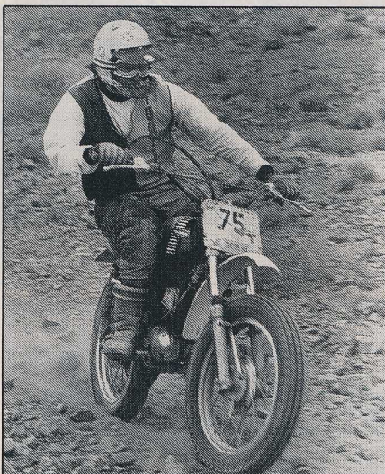
Harley-Davidson hasn't left its mark in the dirt bike world with too many technical innovations, but their Baja 100's foam air filter kept the little bike roosting in conditions that left paper filter-equipped machines of its day dead on the trail.
