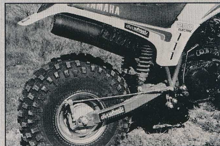
Archaic-looking rear dampers do a superb job of leveling out the nasties. Yamaha uses a jack-shaft arrangement in order for the drive chain to clear the big rear tire.
