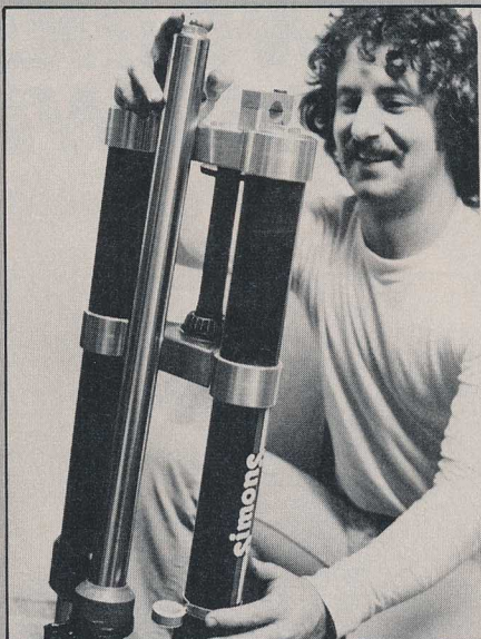
Steve Simons, inventor of the upside-down forks, shows a pair of stock 38mm RM250 forks against the UDX-60s.
