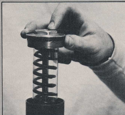
When the fork caps are unscrewed, the springs are lifted with the cap. A clear Lexan tube traps the springs and prevents them from rubbing on the inside of the upper part of the forks.
