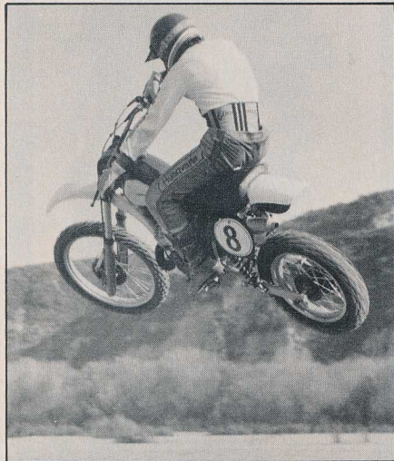
Piggyback Ohlins shocks are mounted outboard of the swingarm, making for easy preload adjustments.
