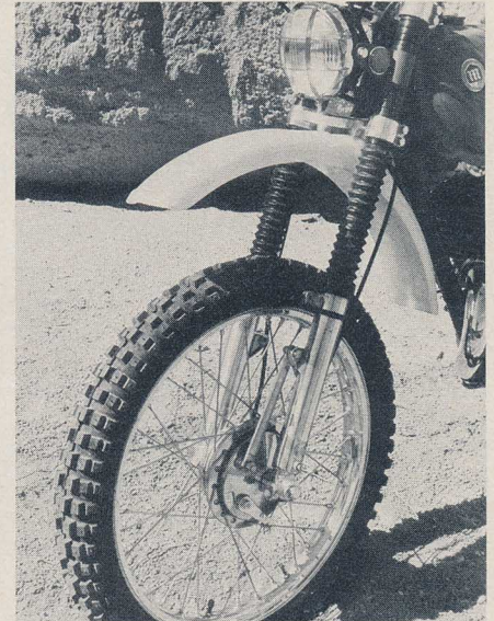
Superb front brake hums a happy tune with Betor fork.
