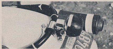
Positive proof that turn signals are good for something. Change the amber to red and hook up the brake light.
