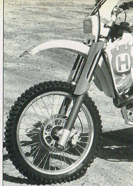
Both the Husqvarna and KTM come with the new 45mm Marzocchi Magnum fork. While the Katoom has stiffer overall settings, Husky's geometry provides a more predictable handling package than KTM. The WXC always feels more planted.
