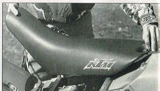
KTM joins the XR600R in having totally toolless air filter access. The LC4 filter is larger than the Honda's, and the airbox is more moto, too.
