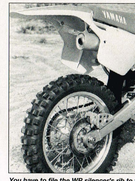
You have to file the WR silencer's rib to fit a spark arrester, and the result is still too loud. Get an Answer Sneaker. The Yamaha rear brake is the strongest of the bunch, but we hate the tire.
