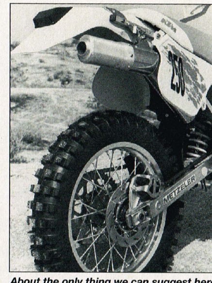
About the only thing we can suggest here is to heat and mold the rear fender under the end of the subframe to provide a handle for lifting, and losing those hideous number plate covers.
