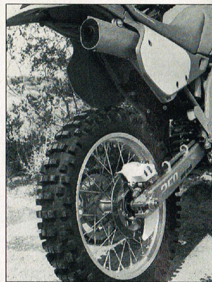
Restrictions apply: The too-choked silencer and too-soft shock put the KDX at a disadvantage at anything more than a snail's pace.
