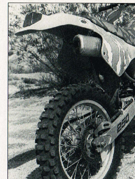
Changes to the rear disc and pad material give more brake life in muddy going. The RMX's M58 loses its edge quickly.
