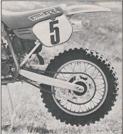
The "works" banana swingarm not only looks wild, it saves some weight and is actually stronger than the stock unit. Ricky Johnson, David Bailey and Gary Bailey all run them on their practice machines. The aluminum chain strengthener keeps the drive chain in line, is lightweight and works. Pro-Circuit's aluminum subframe section shaves some precious weight off the machine and is mondo trick.
