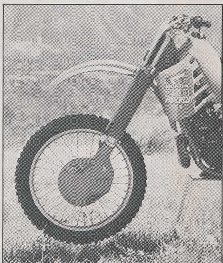
Up front, Pro-Circuit changes the oil to Showa SS-7. These cartridge units are the best dampers on the market. The disc/fork guards are important items; they keep the thin fork legs from getting dented by rocks.
