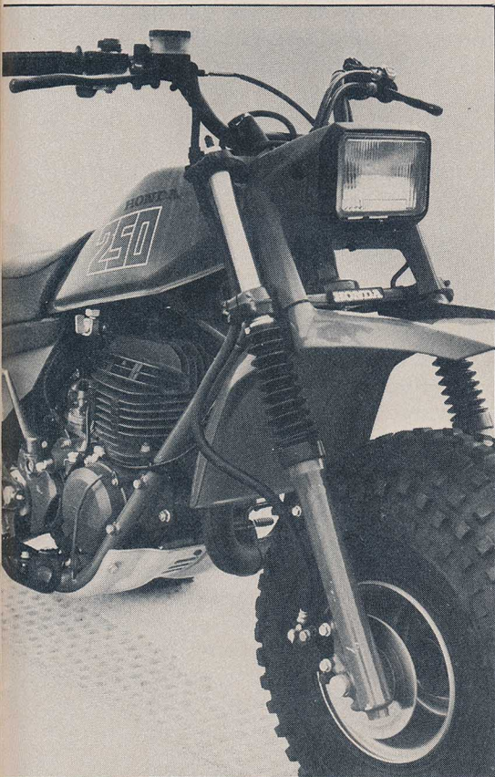
Front forks deliver 6.7 inches of wheel travel. Hydraulic disc brake is a sure stopper—with this kind of power, you need it.
