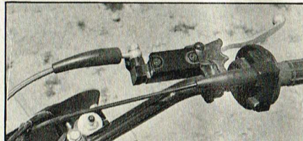
The master cylinder and plumbing for the disc brake is cobby and rather vulnerable. Most riders rig up some sort of guard.
