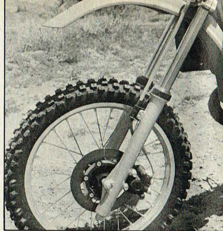
Kawasaki mini riders everywhere love the front disc. For the racing speeds the KX attains, this brake is necessary.
