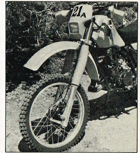
The IT's 43mm forks definitely do the best job in the 200 class. They are plush, strong, and flex-free.
