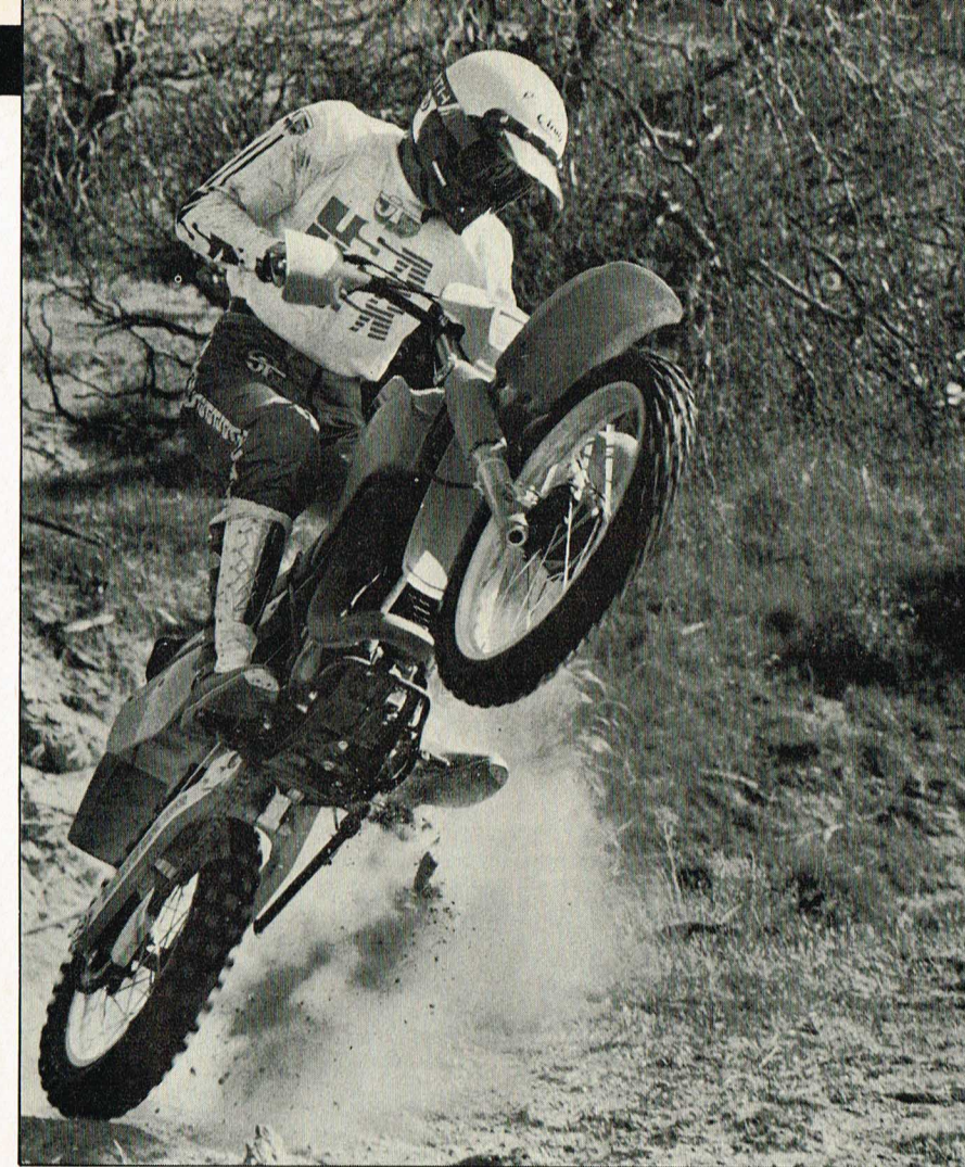
We performed all sorts of acrobatics on the IT. The only "fit" problem we had was with the kickstand. If you have size 10 feet or larger, you can expect your heel to hit the kickstand shaft and cause it to clatter in the rocks while you ride.
