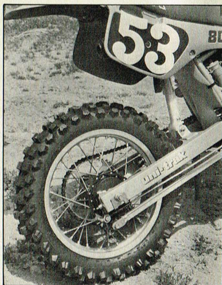
A new swingarm and retuned suspension are improvements for 1985. Our testers praised it for longer travel and a cushier ride.
