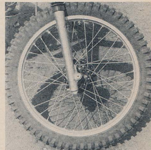
3.00x21 Metzeler on the front end took care of a minor washout problem we had experienced in the past.
