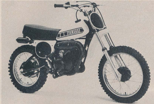
Yamaha YZ80E. First time for Monocross suspension and leading axle forks. Claimed weight 146 pounds. 26 Mikuni. Five speeds.
