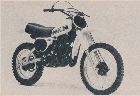
YZ250E. A brand-new, trimmer engine with a sixth gear. Claimed weight 216 pounds. Aluminum swingarm, 38 Mikuni.
