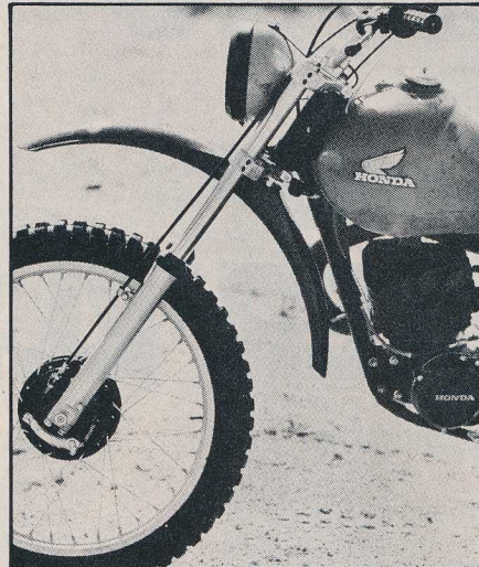
The front end is kicked out for desert stability.
