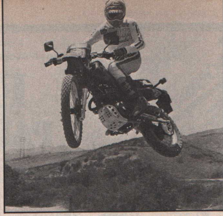
It IS possible to cross up the XL600, but it's not comfortable. When it landed, the rear brake actuating lever would hit the muffler.
