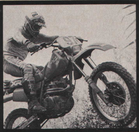
Aluminum alloy abounds on the WB Honda, with a Megalloy muffled silencer and a trick swingarm. Engine mods were basic but effective enough to add nine ponies to the mild stocker.
