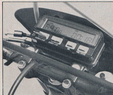
Honda's odometer/clock combo is sophisticated piece of enduro equipment that's easy to set and adjust, and can even be calibrated to mileage markers used in enduros.
