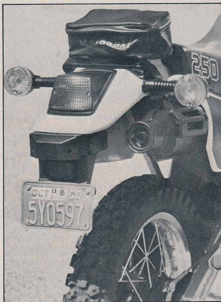
A quiet spark arrester/muffler, good-sized tool pouch, flexible turn signals and integral taillight ride at the rear of the KLR. Both front and rear fenders are plastic, but the fuel tank is metal.
