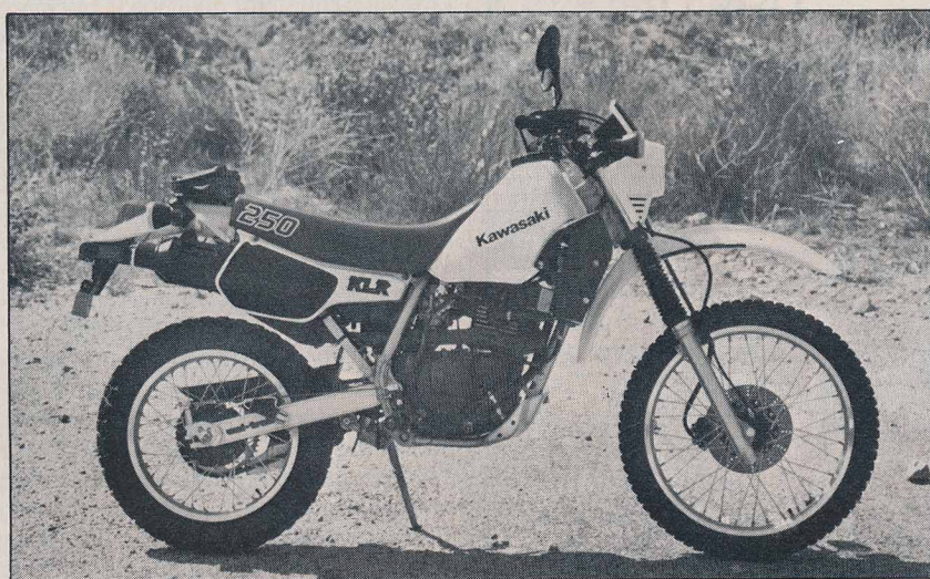
A quiet spark arrester/muffler, good-sized tool pouch, flexible turn signals and integral taillight ride at the rear of the KLR. Both front and rear fenders are plastic, but the fuel tank is metal.
