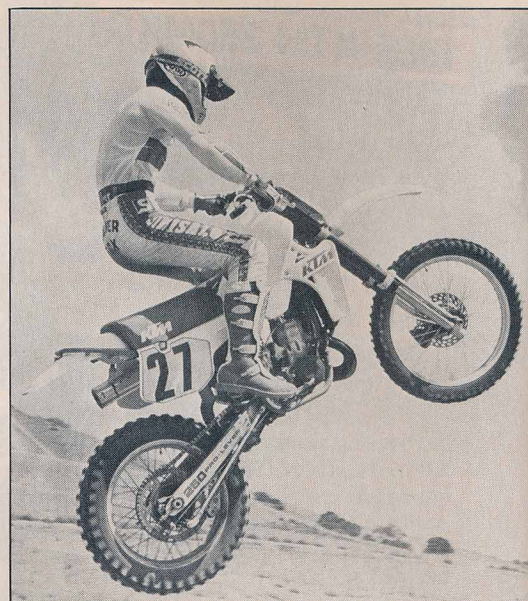
We found the rear suspension able to soak up any kind of an impact, even rear wheel landings from a surprising altitude. One-hundred-and-fifty-pound riders may feel the need for a softer spring.
