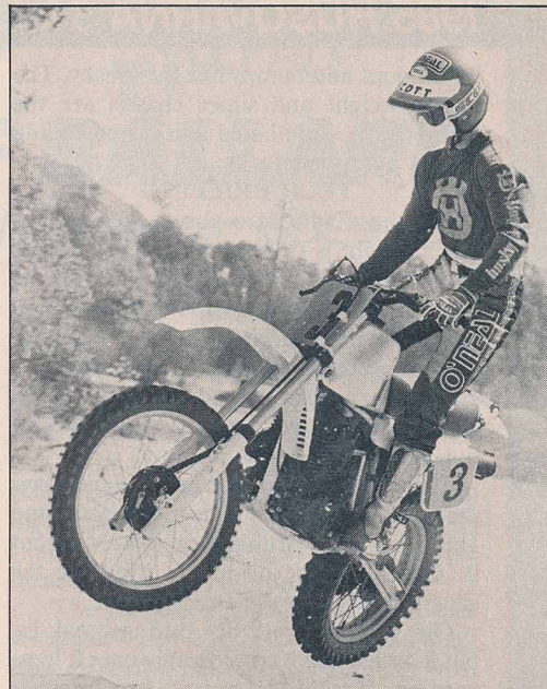
Just-right forks and too soft shocks left the stock bike a bit unbalanced.
