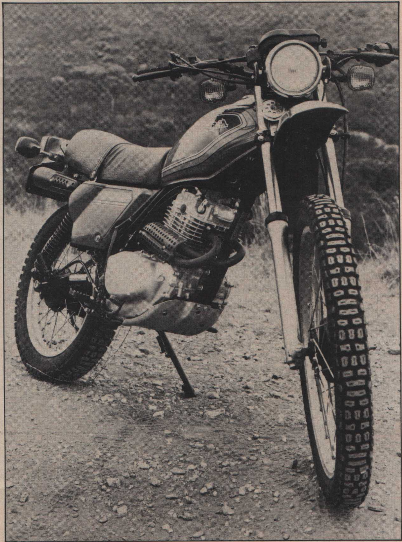
Weak point of both bikes is a set of spindly forks. Claw action tires are a decent compromise, but wear fast.
