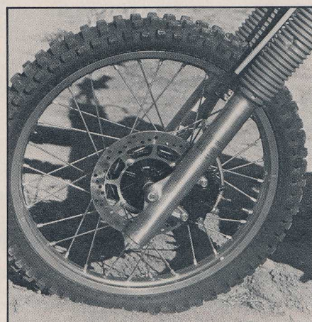
One of the finest stoppers in the land can be found here. Brake action is super strong, yet predictable.
