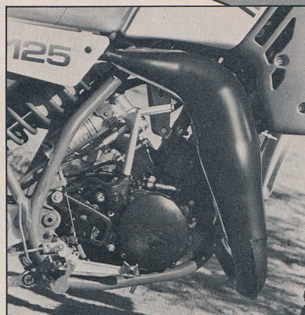
Revised pipe and porting increase the power over the 1984 model, but not enough. Close, but no hand grenade.
