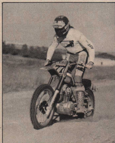
With almost 14 inches of travel in the rear, the HPF Honda would soak even the toughest terrain.
