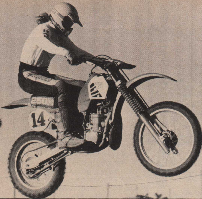
Twin radiators are very light and mount on each side of the tank. Plastic scoop on sides directs air to radiators; they fold in easily if the bike is dropped, then spring back into shape.
