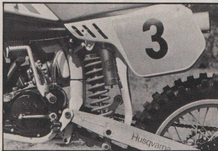
A superb Ohlins shock does 13-plus inches of impeccable travel work. Both adjusters for the damping are external.
