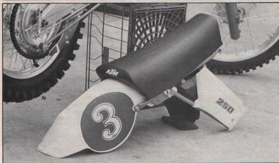
Since the entire rear section of the frame unbolts, shock maintenance is a cinch.
