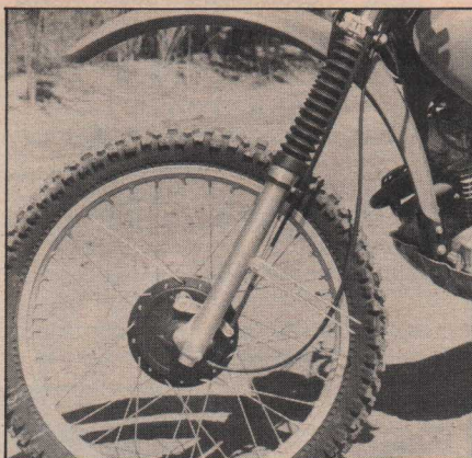
Both front ends are identical, with 23-inch wheels and 8.8 inches of travel.
