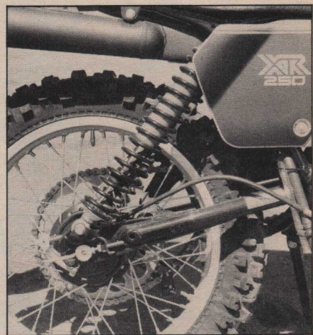
XR250 rear end has all the same numbers as the 500, but the backing plate is anchored by a boss on the swingarm, rather than the torque arm of the latter.
