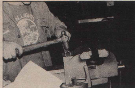
Hammering on each side of the split will partly close it.
